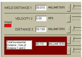
The section to the left shows the window as it would be displayed for a typical setting. It will only be displayed if Distance 2 has a non-zero value, incremental weld mode is selected and one of the distances has been given the focus as described above.
